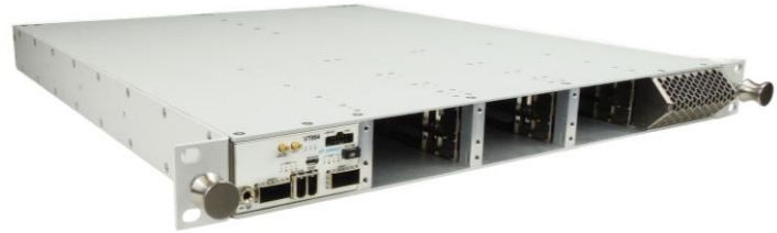
Figure 1: VT954 Chassis Front View
