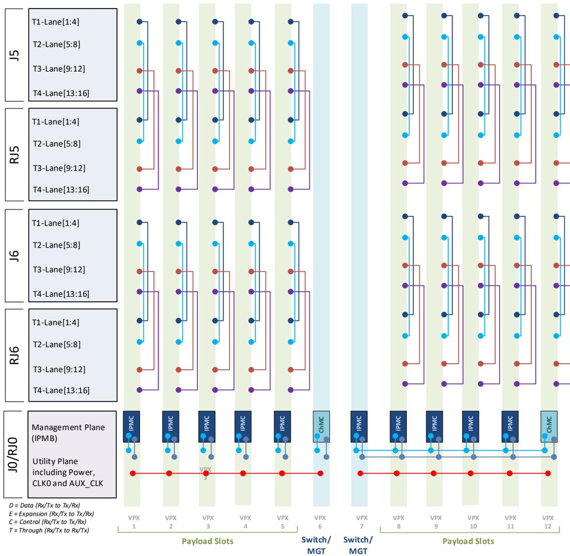
Figure 4: VTX866 Backplane Connections J5-J6 and J0
