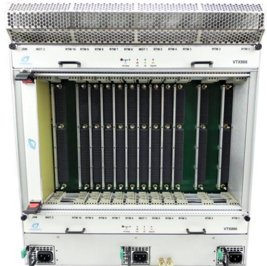
Figure 2: VTX866 Rear View
