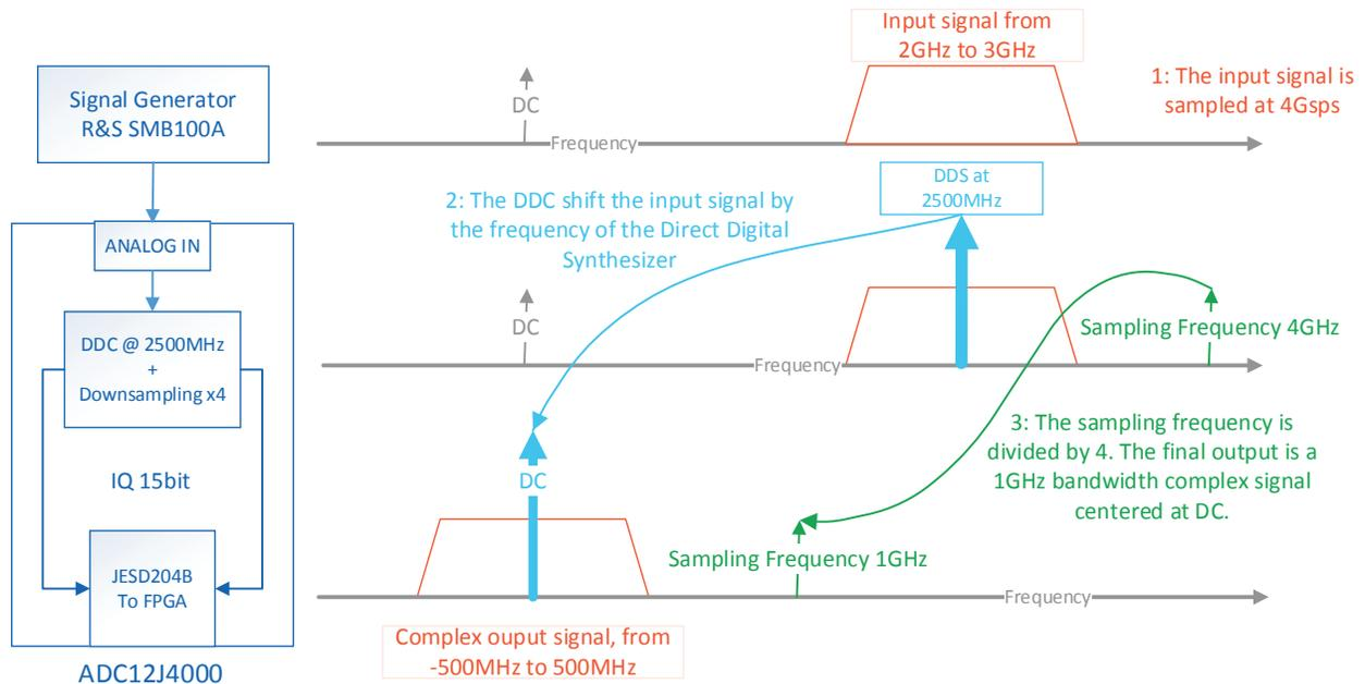
**Figure 3:** ADC12J4000 Digital Down Converter
