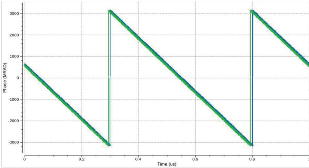
**Figure 21:** Input phase after ADC Sampling clock adjustment
