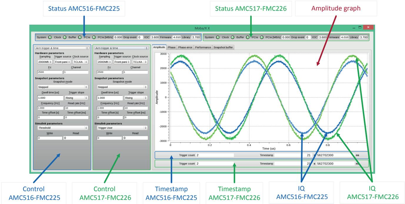
**Figure 4:** DAQ Series dual channel GUI
