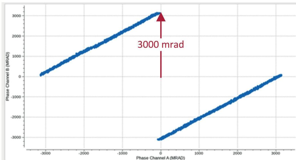
**Figure 18:** Phase error before adjustment
