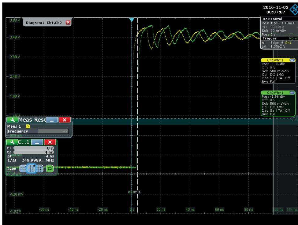
Figure 14: Sampled trigger signal before adjustment
