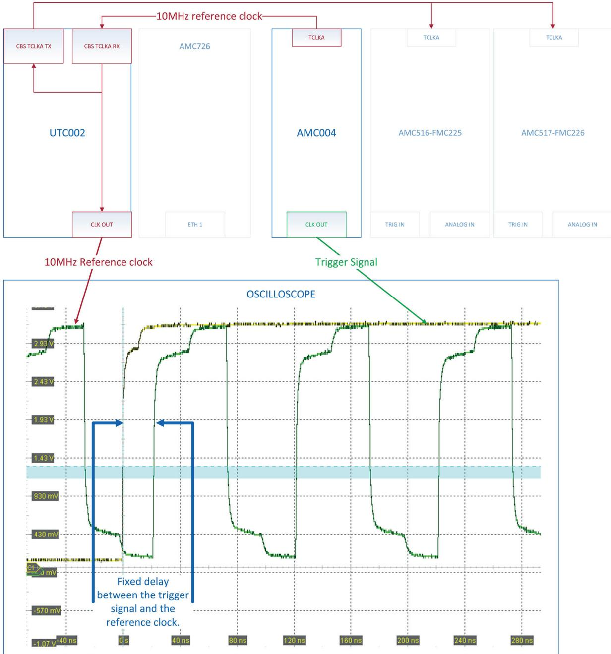
**Figure 2:** Deterministic delay between AMC004 trigger and 10MHz clock
