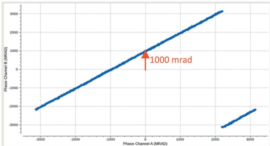
**Figure 20:** Phase error after sysref adjustment
